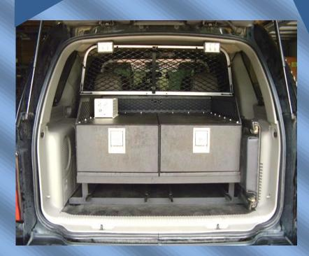
14- Gauge reinforced powder coated steel
